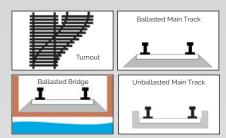
KLP® Hybrid Polymer Sleepers are ideal for ballasted track, for example, in the application of switches and crossings. The elasticity of the polymer provides good damping and reduces wear. The steel bars, that are completely encased within the KLP® Hybrid Polymer Sleeper, reinforce the sleeper and also optimize its stiffness.
